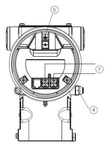
1 Power source | 2 Remote indicator | 3 Handheld communicator | 4 External ground termination point | 5 Internal ground termination point | 6 Line load | 7 Fieldbus line (polarity independent)
