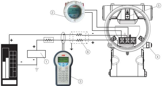
HART hand-held communicator may be connected at any wiring termination point in the loop, providing the minimum resistance is 250 ohm. If this is less than 250 ohm, additional resistance should be added to allow communications. Maximum voltage drop on external remote indicator is 0.7 V DC.
