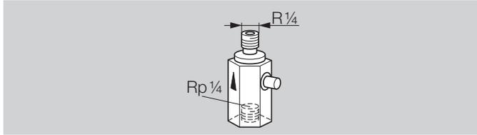
To test the pressure switch, the DG can be vented using the PIA test key (contains non-ferrous metals).
