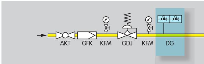
If the pressure is either too low or too high, the min./max. pressure switch DG switches in order to avoid start-up or to initiate a safety shut-down.
