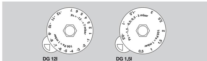
In the negative adjusting range, the template which can be found in the unit displays the connection diagram.
