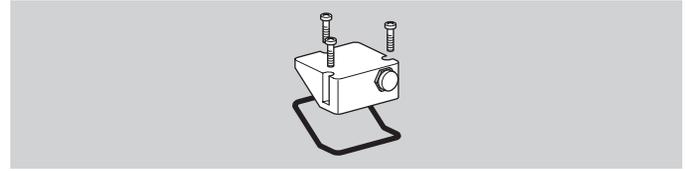
To avoid the formation of condensation, the cover with pressure equalization element can be used. The diaphragm in the screw connector is designed to ventilate the cover, without allowing water to enter.
