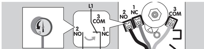
DG..B, DG..U und DG..H switch with rising pressure. The contact switches from NC 1 to NO 2.
