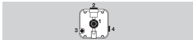
Ports 3 and 4 are connected to the upper diaphragm chamber. To prevent the micro switch from being damaged, no pipe conducting a gas/air mixture may be connected. Air and flue gas may not contain any aggressive constituents.
