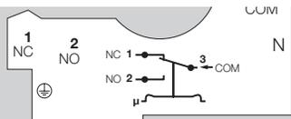
Contacts 3 and 2 close when subject to increasing negative pressure. Contacts 1 and 3 close when subject to falling negative pressure.
